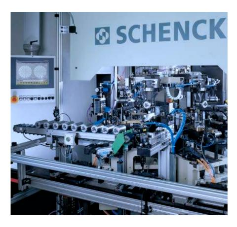
Integrated overhead rotary transfer machine
