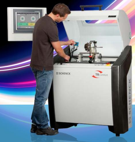
The **TB**comfort creates the basis for a high-quality overhaul: In the first step the initial unbalance of the components is removed and the mounted rotor assembly is secured. This creates the requirement for subsequent high-speed balancing. This process is made easy by the simple and logical operation of the **TB**comfort, the ergonomic design of the complete system and its high precision. For example, the easy mounting of the rotor in the machine with
