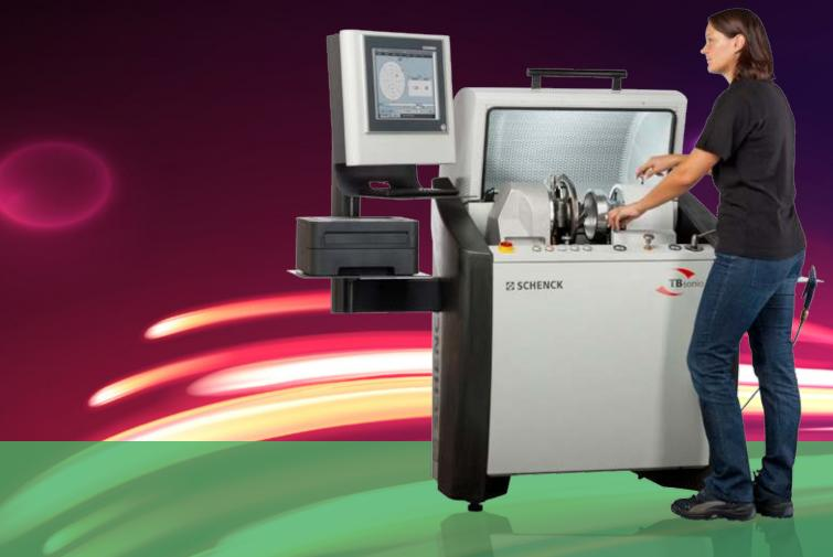
Low-vibration – at the end of the overhaul process the core assembly is accelerated with compressed air on the **TB**sonio and is then balanced under largely realistic conditions. Only after this process does the turbocharger have such a low residual unbalance that it reaches a quality level comparable with a new turbocharger.
